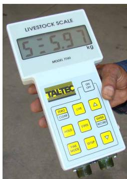
1. The instrument is powered by a 6 volt (lead acid sealed) battery and not mains. If the battery is low it will affect the performance of the scale. Charge the battery using the Mains adaptor or Car battery jumper lead both supplied with a new scale.
