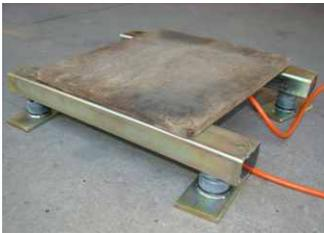
1. (Back ground) Each loadbar is fitted with two loadcells. There is an electric current flowing through each loadcell. When an animal stands on the scale there is a resistance change in the loadcell; this change is in the range of millivolts. So if there is any damage to the cable, plugs or loadbar the instrument is reading that damage and displaying an in-correct mass.
