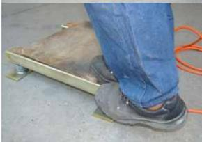
5. If not, identify the loadbar with the problem (the one with the incorrect reading). Inspect the loadbar for cable damage; loose bolts or a shifted loadcell or plug damage. Repair yourself or return to Tal-Tec.
