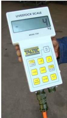
3. Switch the instrument on. Now connect the plug from the loadbar; one at a time; after each one observe the reading on the display; the reading should be less than  $\pm 100\text{kg}$  and stable. This reading is called the offset and is normal. If the offset is above 100kg it is possible that a loadcell has been overloaded. If the offset is fluctuating in the hundreds it could indicate water damage. If the offset is fluctuating in the thousands it could indicate cable damage.
