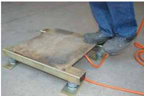
now climb off. The display must return to zero. Now repeat this on every corner; remember to climb off every time. If the readings are the same on every corner your scale is in a good condition.
